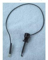
The flying tap lead is created using the test clip lead with crimp terminal placed on the end and covered with heat shrink tubing.
