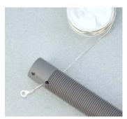
Next, install the end caps into the PVC tube and secure with 2 screws and washers on the same side of the coil as the lengthwise slot.
