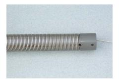
Continue winding to the other end of the tube until you have reached the end of the threaded area of the form. It is important to wind all the way to the end of the threaded area as this ensures sufficient number of turns on the coil.
